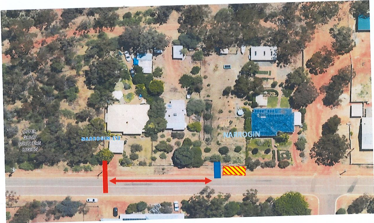
Figure 3 Showing approximate position of blind crest and 50 metre distance to driveway area
