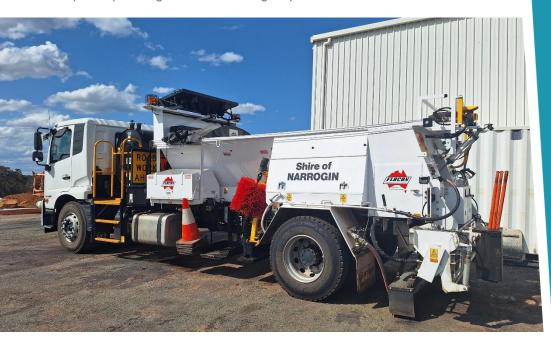
Let our Jet Patching truck repair those nuisance pot holes on your road network minor rut corrections or even seal or re-seal lengths of road that need renewal.
